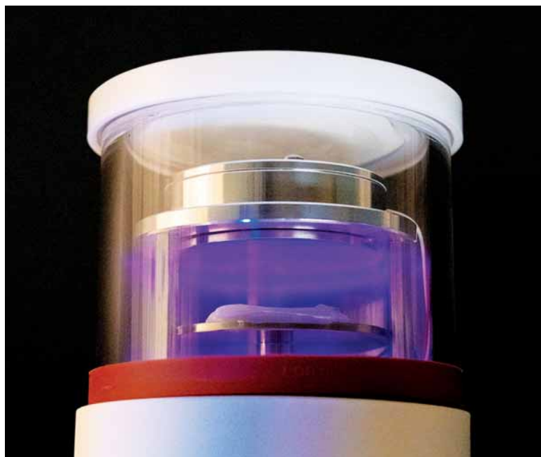
The Darst and Bonilla labs utilize glow discharge systems to prepare samples for advanced structural imaging.
