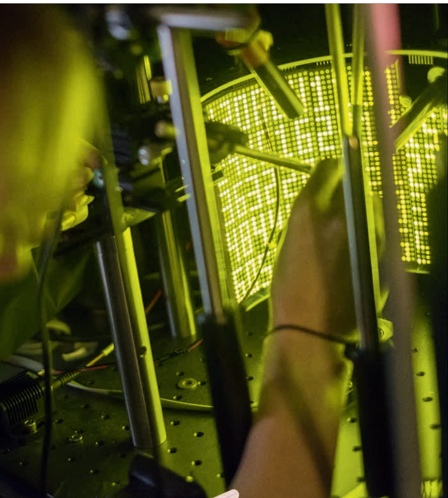
In Maimon's lab, scientists use panels of LEDs to create a virtual reality environment for fruit flies.
